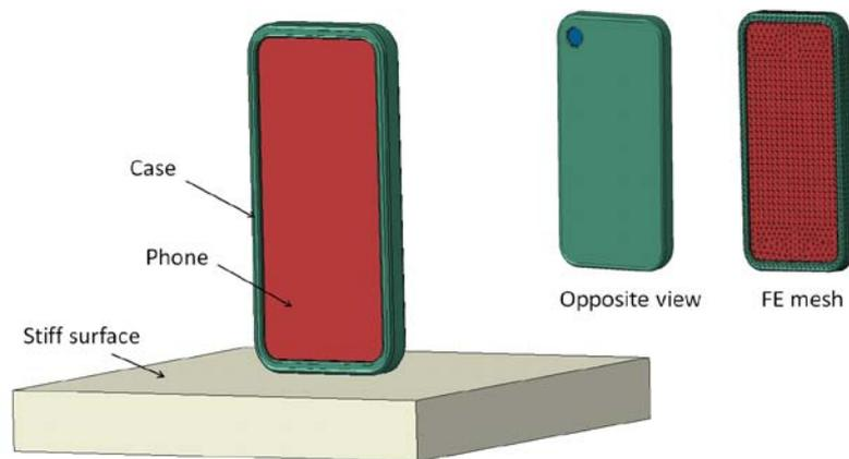
**Figure 6:** Model and finite element mesh used for the phone drop test.
