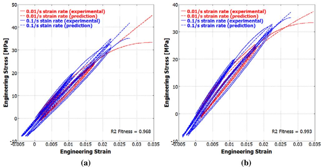
**Figure 4: Comparison between experimental results and (a) linear viscoelastic material model and (b) Parallel Network Model for Material 1.**
