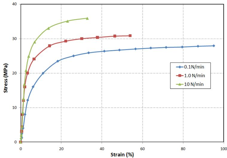
**Figure 2:** Engineering stress-strain curves for Material 2 (plasticized PLLA) at three loading rates. Data from Grabow et al. (2005).
