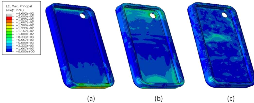
**Figure 7:** Maximum principal strain contours at (a) 0.1 ms, (b) 0.18 ms, and (c) 0.48 ms.
