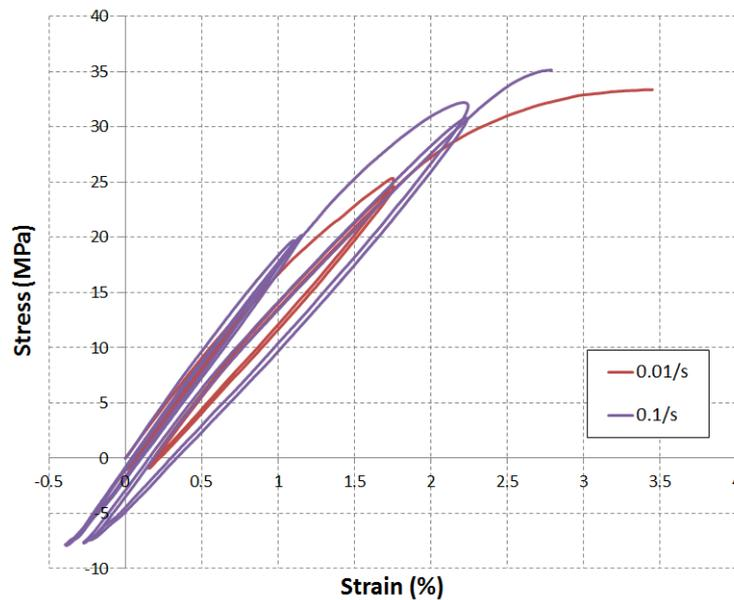
**Figure 1:** Engineering stress-strain curves for Material 1 (a pure PLA) subjected to uniaxial tension load-unload cycles at two strain rates.
