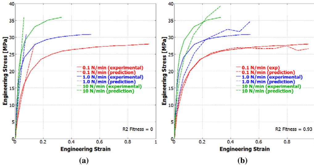
Figure 5: Comparison between experimental results and (a) viscoelastic material model and (b) Parallel Network Model for Material 2.
