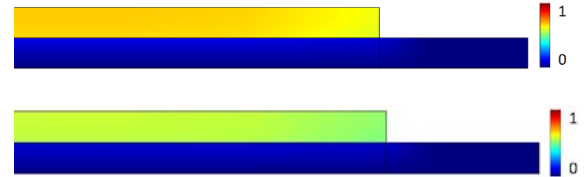
Figure 3. Normalized drug concentration after 60 hours. Top figure without enhancer, Bottom figure with enhancer. Initial enhancer concentration is 0.12 g/cm 3
